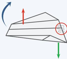
When you put paperclips on the back of the airplane, the center of gravity moved farther back. This extra weight pulls the back of the plane down, while the center of lift pulls the front up. The airplane is unstable!
