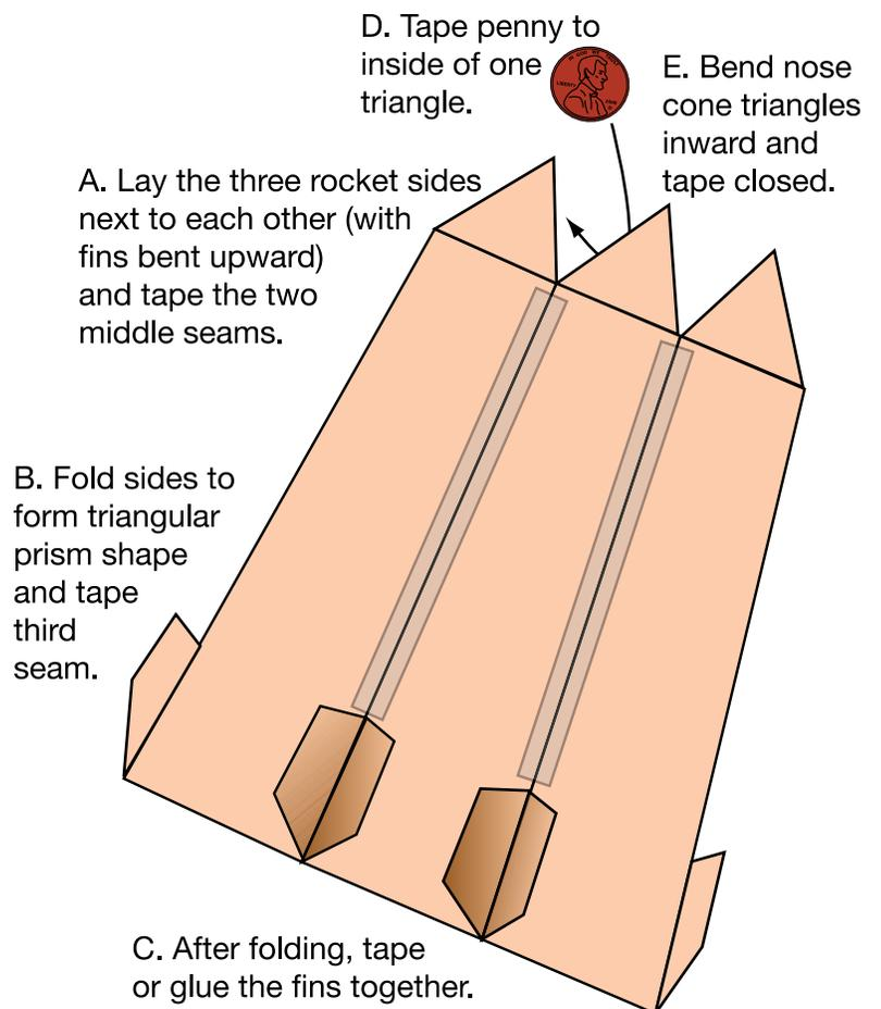
5. Tape a penny securely to the inside of one of the nose cone triangles.
